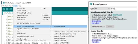
Ensure that the board package (Arduino MegaAVR Boards) for Arduino Nano Every is installed. To check, click on Tools > Board > Boards Manager and search for "Every" as shown above. If required, click on the 'Install' button to install the board package.
